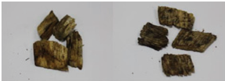
Figure 2. Macroscopic morphological changes of the oak chips subjected to rapid heating and pressure treatment(left: untreated, right: heat-treated)
